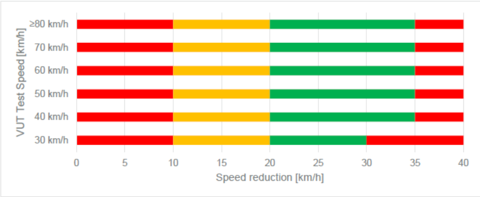
Figure 5-2 Speed Reduction colour band criteria (applicable to Car & PTW Front)
